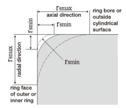
rs min=smallest permissible single chamfer dimension (minimum limit)
